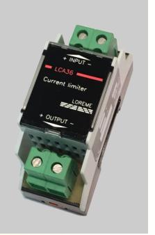
The LCA36 is a inrush peak current limiter for capacitive load. It works like a current clamping circuit, it limits the peaks of current in the load when starting installations.
